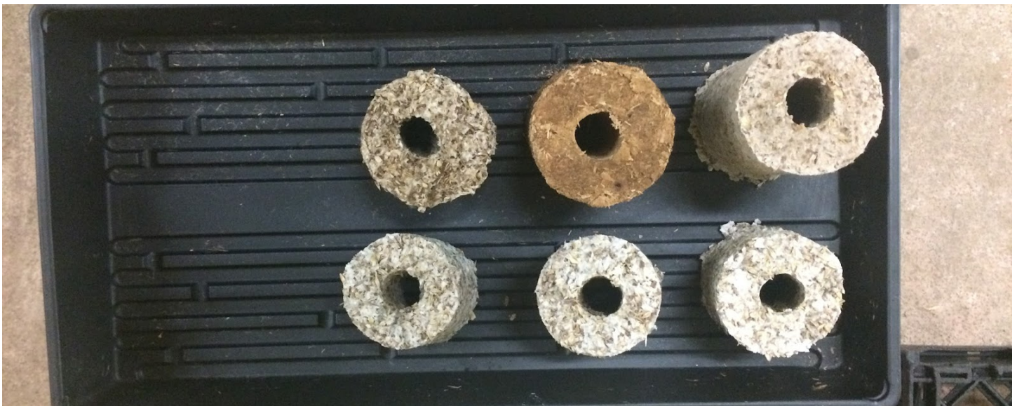
Image 3: Hollow Cylinder Briquettes (Top row, from left to right: 50% grain and sawdust - briquette type 3, 100% sawdust - control sawdust briquette, 50% milled grain and sawdust - briquette type 6. Bottom row: 50% grain and paper pulp - briquette type 5)
