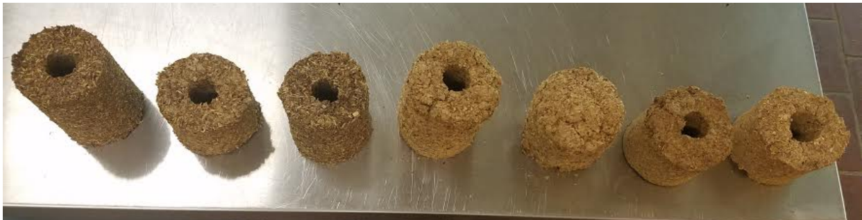
Biobricks from a variety of mixtures and molds (from left to right): 50/50 milled grain and chaff (first 2), 65/35 milled grain and chaff, 100% whole chaff, 100% whole chaff from solid cylinder mold, 100% milled chaff, 50/50 milled chaff and sawdust.
