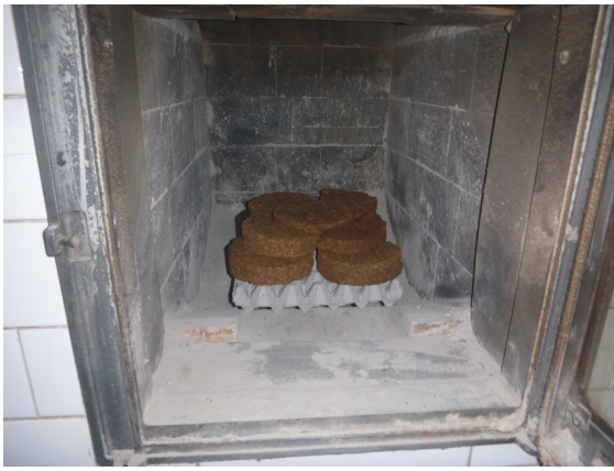
Biomass Briquettes in the auxiliary oven
